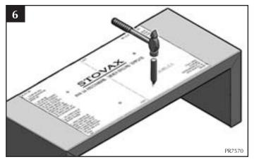
6. Mark drilling points with a centre punch.
